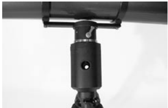
Figure 8. The optical tube must be at a 90° angle to the R.A. axis in order to view through the polar axis finder.
